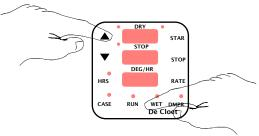
If operating in delta T Hold the "WET" button down and at the same time press an arrow key until the desired new temperature is displayed.
