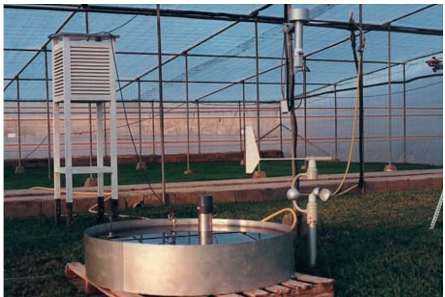
Precipitation meter for the mechanical acquisition of the precipitation for determining the water entry, e. g. in soil, artificial lakes, ponds etc.
