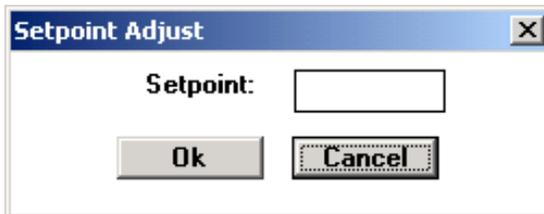
The Set Point Adjust Option allows changing the PXR Controller Set Point. To change the Controller Set Point, enter the desired Set Point. Select "OK."
